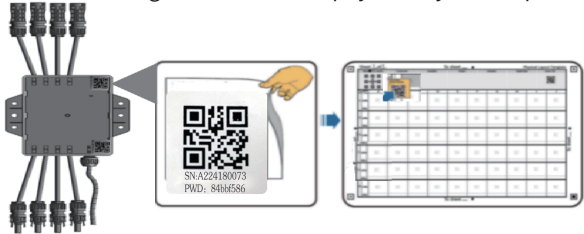
f. Schematic diagram of optimizer concentrator QR code tearing and pasting
