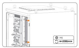
Figure 11-1 Removing the alignment plate
