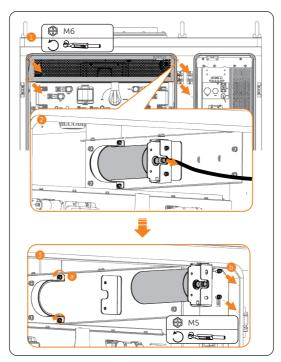
Figure 22-2 Removing the automatic fire sprinkle
