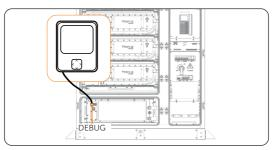
Figure 5-5 Connecting the filed communicator
