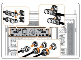
Figure 6-1 Removing the cables
