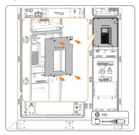
Figure 9-1 Removing the panel
