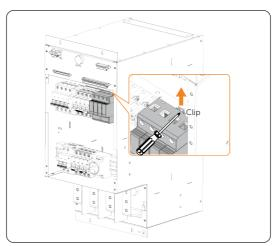
Figure 16-6 Removing the SPD module
