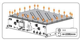
Figure 6-10 Removing the upper cover
