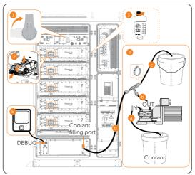
Figure 25-7 Coolant filling
