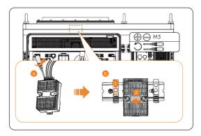
Figure 14-1 Removing temperature and humidity sensor
