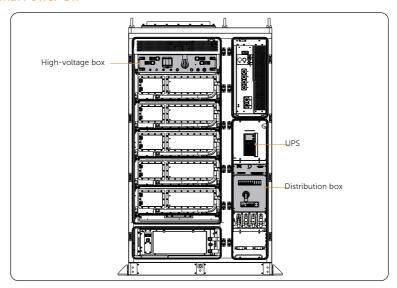
Figure 3-1 Position of modules for normally powering off system
