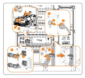
Figure 5-1 Removing cables and pipes of battery pack
