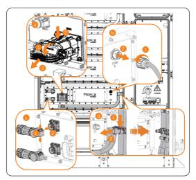
Figure 5-6 Removing cables and pipes
