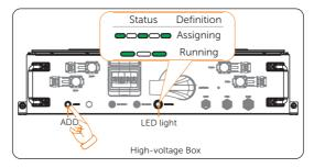
Figure 6-9 Assigning the address
