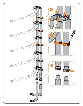
Figure 23-4 Removing the cabinet pipe
