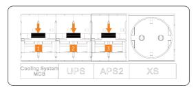
Figure 3-3 Flipping down breakers on distribution box (1)
