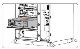
Figure 5-3 Installing the new battery pack
