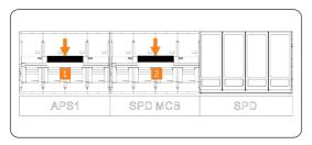
Figure 3-4 Shutting down breakers on distribution box (2)
