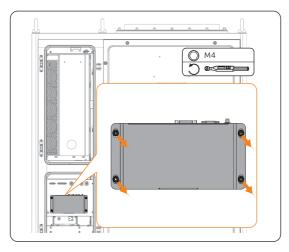
Figure 7-2 Removing the EMS
