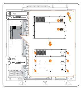
Figure 17-1 Removing the dehumidifier
