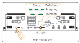
Figure 6-3 Assigning the address
