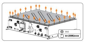
Figure 6-7 Removing the upper cover
