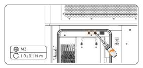
Figure 13-2 Installing a new door sensor.
