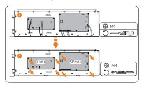
Figure 6-5 Removing the HVU or SBMU (Left view)
