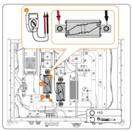
Figure 6-8 Removing the faulty fuse (Top view)
