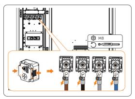
Figure 16-2 Removing the cables
