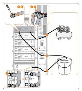
Figure 25-6 Draining the coolant
