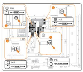
Figure 6-12 Removing contactor (top view)
