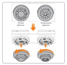
Figure 12-1 Removing the detector
