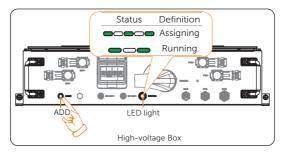
Figure 5-4 Assigning the address
