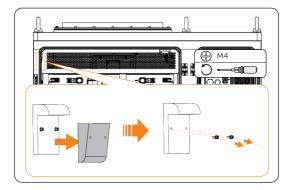
Figure 19-1 Removing the audible and visual alarm
