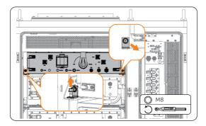
Figure 6-2 Removing the faulty high-voltage box
