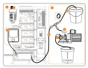
Figure 25-5 Coolant filling
