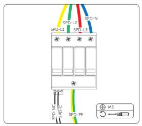
Figure 16-5 Removing the cables of SPD module
