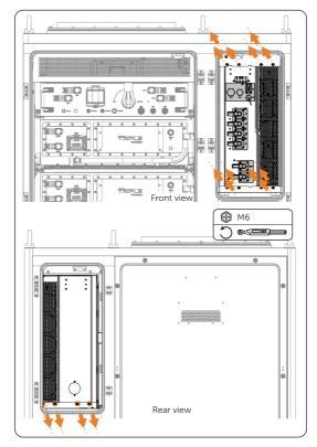
Figure 20-1 Removing the PCS
