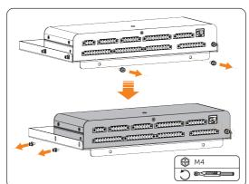
Step 3 Remove the IO module from the cabinet and the bracket.
