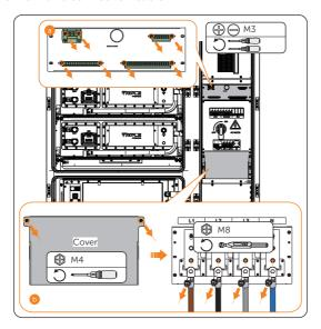
Figure 16-1 Removing the cables
