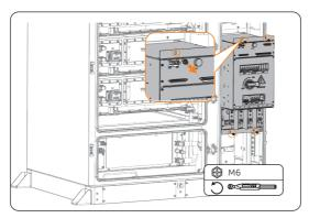
Figure 16-3 Removing distribution box
