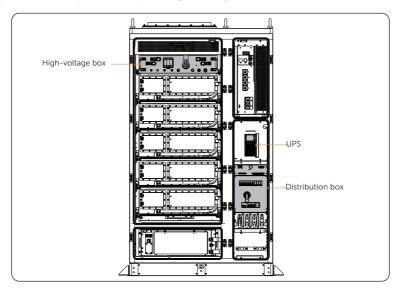
Figure 3-10 Position of modules for powering on system
