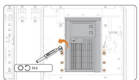
Step 3 Unscrew the screws that fix the UPS and take out the UPS.
