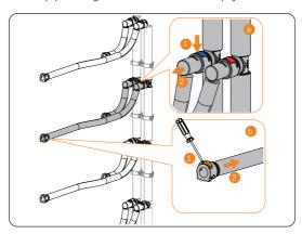
Figure 23-3 Removing the battery pack pipe
