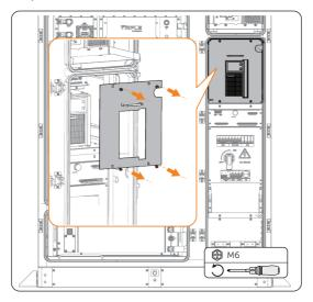
Figure 10-1 Removing panel
