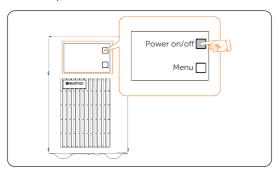
Figure 3-8 Shutting down the UPS
