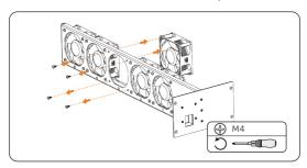
Figure 20-3 Fan remove
