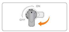
Figure 3-11 Switching on the distribution box
