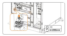
Figure 5-2 Taking out the battery pack
