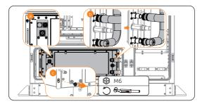
Figure 21-1 Removing the liquid cooling unit
