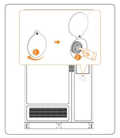
Figure 3-9 Pressing emergency stop button
