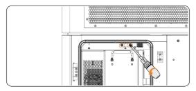
Figure 13-1 Removing the door sensor
