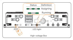
Figure 6-14 Assigning the address
