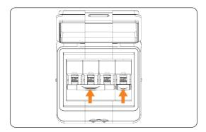
Figure 3-15 Flip up breakers on high-voltage box
