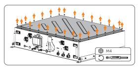
Figure 6-4 Removing the upper cover
