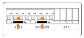
Figure 3-12 Flipping up breakers on distribution box (1)
