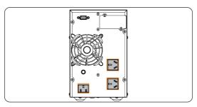
Figure 9-2 UPS Wiring Panel
