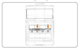
Figure 3-7 Flipping down high-voltage box breakers
