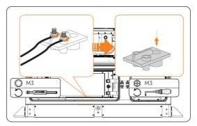
Figure 18-1 Removing the water sensor
