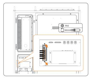
Figure 8-1 Removing the Switch
