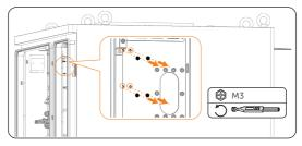
Figure 11-3 Removing CO detector
