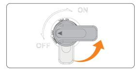
Figure 3-5 Switching off the distribution box
