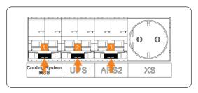
Figure 3-13 Flipping up breakers on distribution box (2)
