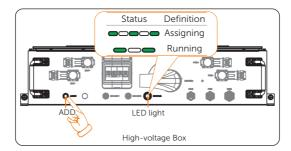
Figure 5-8 Assigning the address
