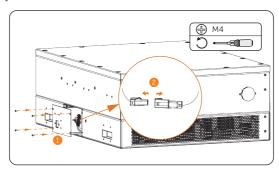
Figure 20-2 Disconnecting the fan
