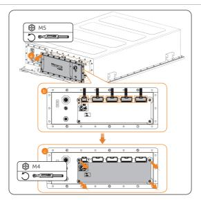
Figure 5-7 Removing the PCBA
