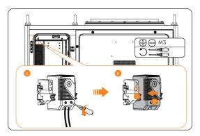
Figure 15-1 Removing the thermostat
