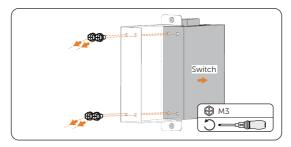
Figure 8-2 Removing the Switch
