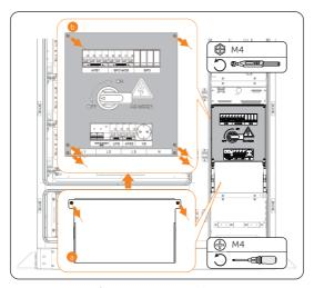
Figure 16-4 Removing the front panel
