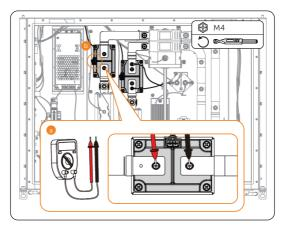
Figure 6-11 Removing the cables
