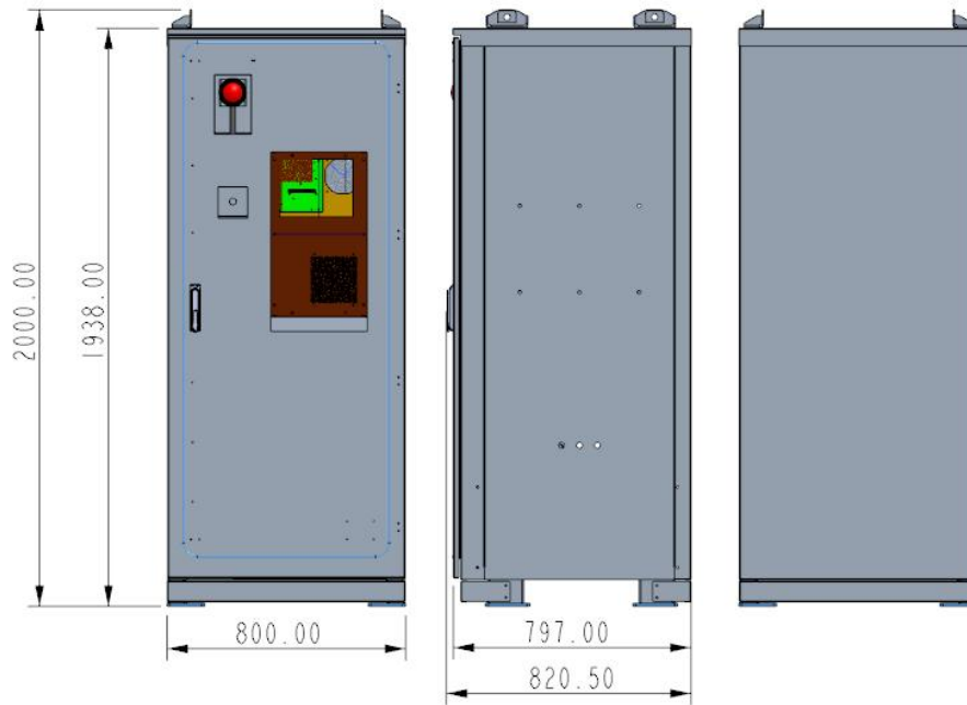
Figure 5-1 Machine Dimensions Overview
